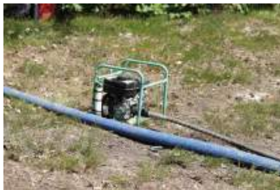
Figure 82. Pompe thermique. Photo ©CDPNE
